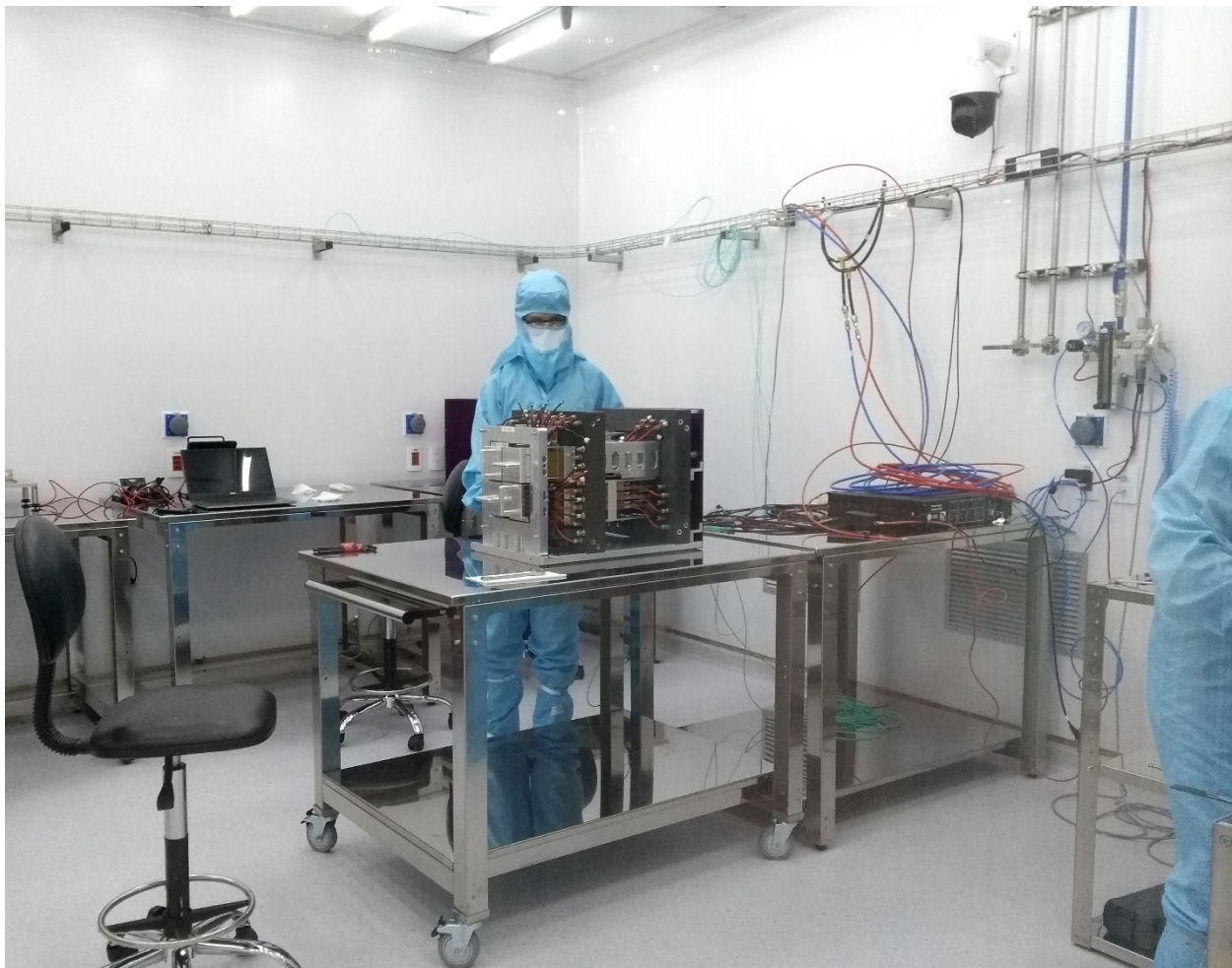
Assembling PIMEGA 540D #2 detector for SAPUCAIA beamline
